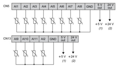
(1) (CN5 + CN13) Max. current : 50 mA. (2) (CN5 + CN13) Max. current : 150 mA.
